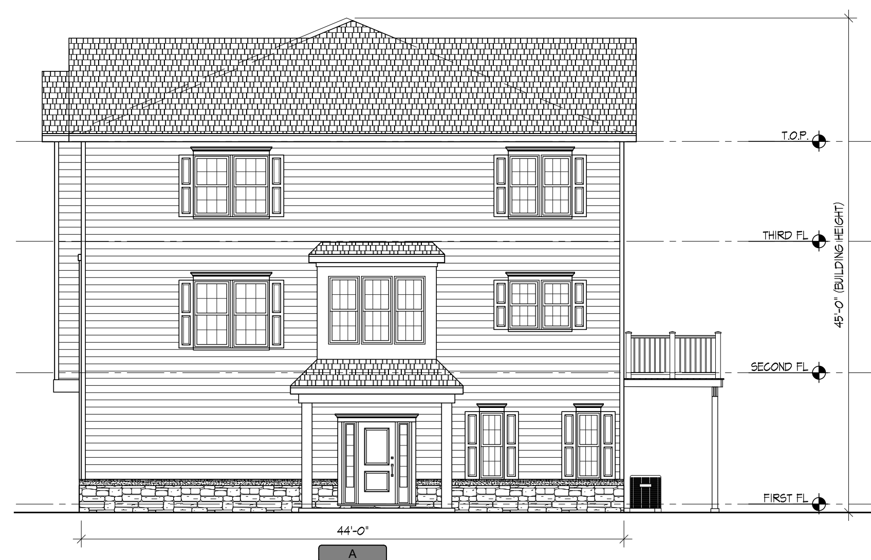
4 7-UNIT BUILDING (STYLE 1) - RIGHT ELEVATION SCALE: 1/8" = 1'-0"
