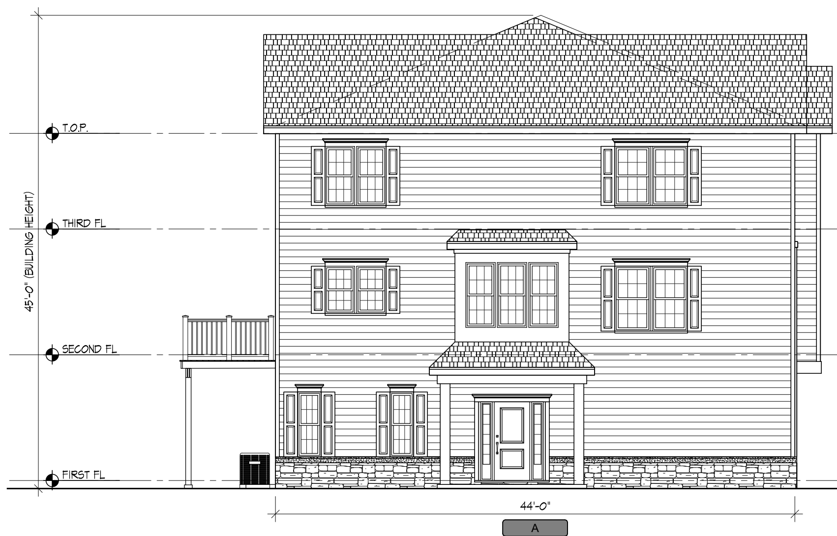
3 6-UNIT BUILDING (STYLE 2) - LEFT ELEVATION SCALE: 1/8" = 1'-0"
