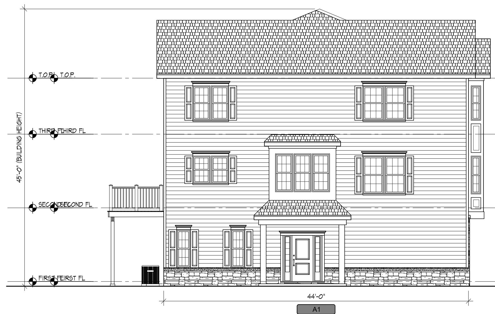
3 7-UNIT BUILDING (STYLE 2) - LEFT ELEVATION SCALE: 1/8" = 1'-0"
