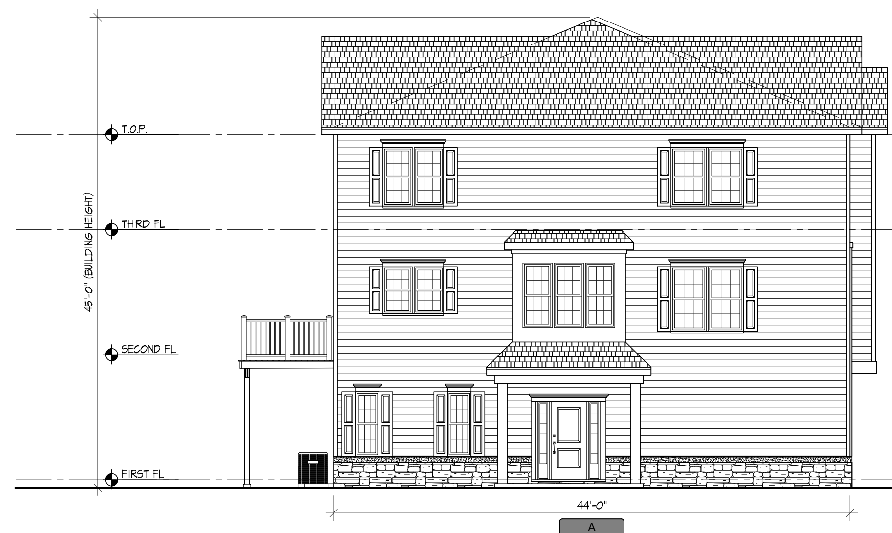
3 7-UNIT BUILDING (STYLE 1) - LEFT ELEVATION SCALE: 1/8" = 1'-0"
