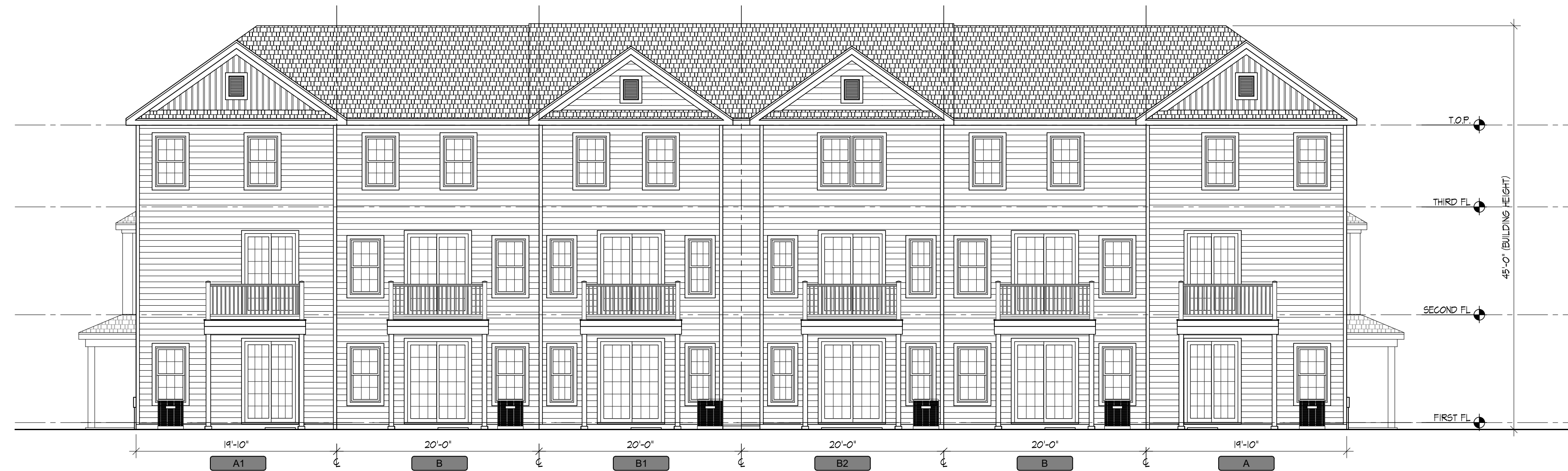
2 6-UNIT BUILDING (STYLE 2) - REAR ELEVATION SCALE: 1/8" = 1'-0"
