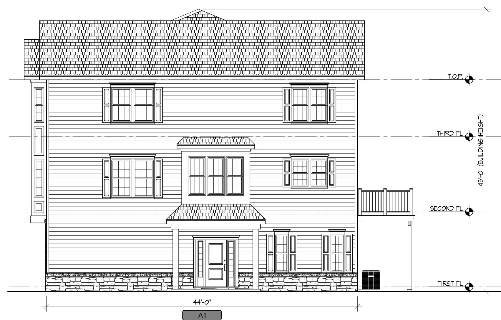
4 6-UNIT BUILDING (STYLE 2) - RIGHT ELEVATION SCALE: 1/8" = 1'-0"
