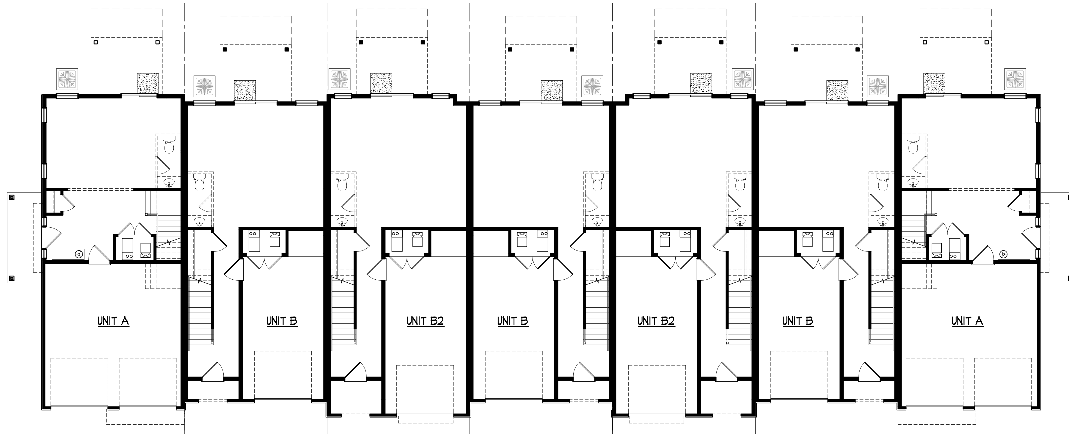
7-UNIT BUILDING (STYLE 1) - FIRST FLOOR SCALE: 1/8" = 1'-0"
