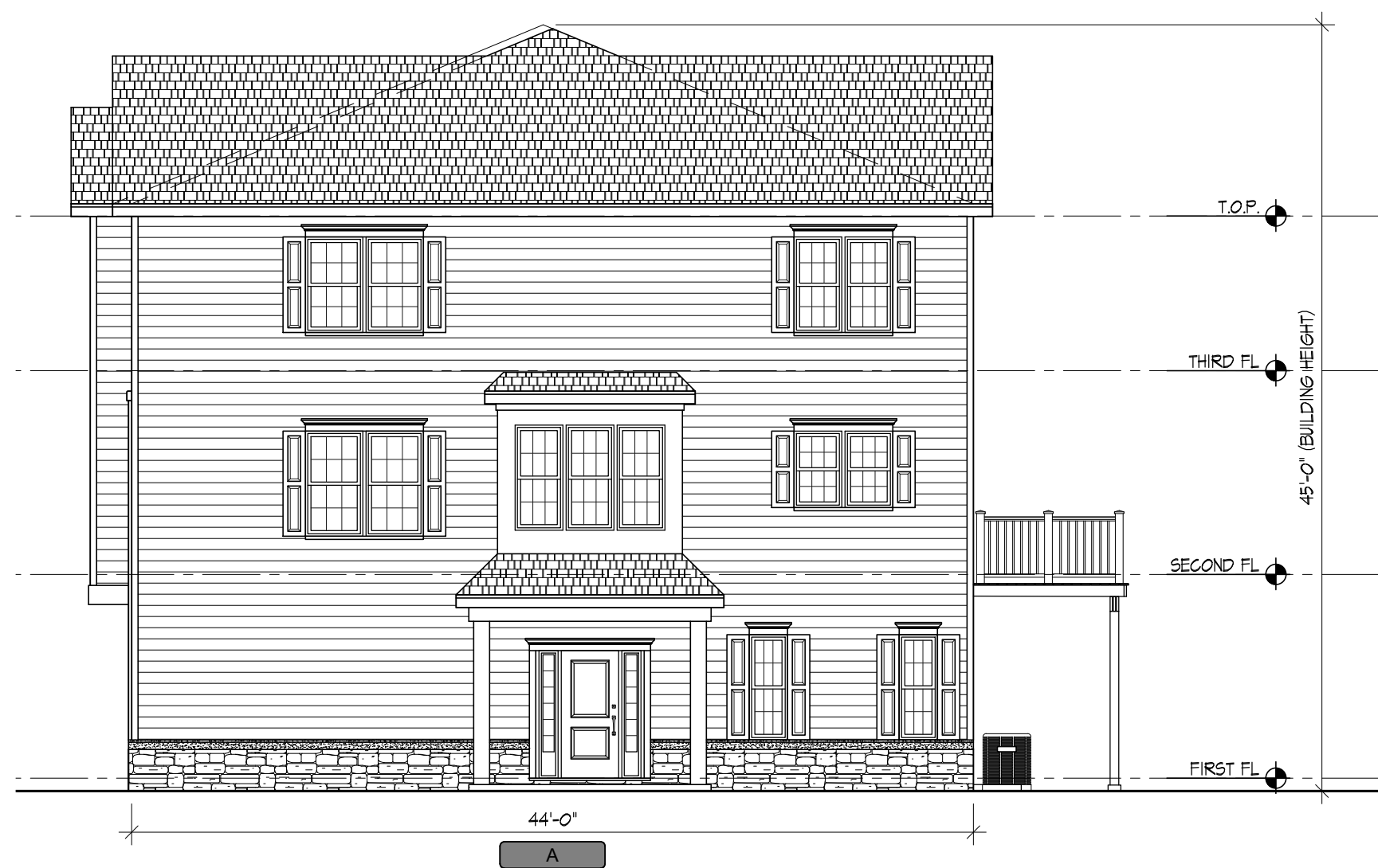
4 8-UNIT BUILDING (STYLE 1) - RIGHT ELEVATION SCALE: 1/8" = 1'-0"
