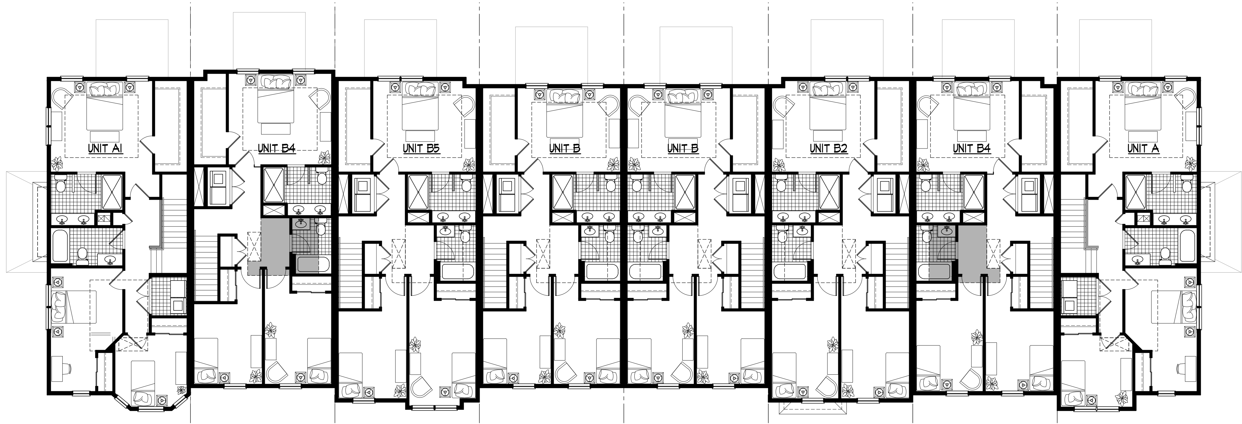
8-UNIT BUILDING (STYLE 1) - THIRD FLOOR SCALE: 1/8" = 1'-0"
