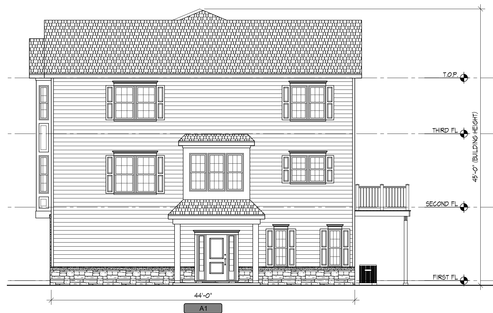
4 7-UNIT BUILDING (STYLE 2) - RIGHT ELEVATION SCALE: 1/8" = 1'-0"
