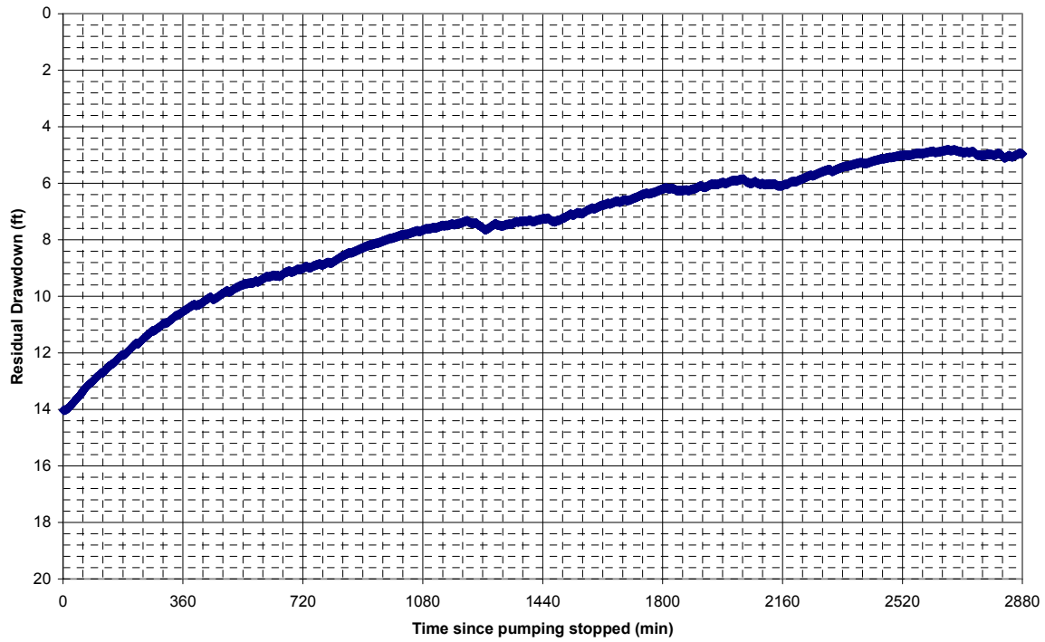
Figure 16: Water Levels in Piezometer 1 After Pumping Well 2
